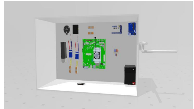
Figure 3: Electronic box with the main components: Jetson Tx2, Pixahawk, Arduino uno
